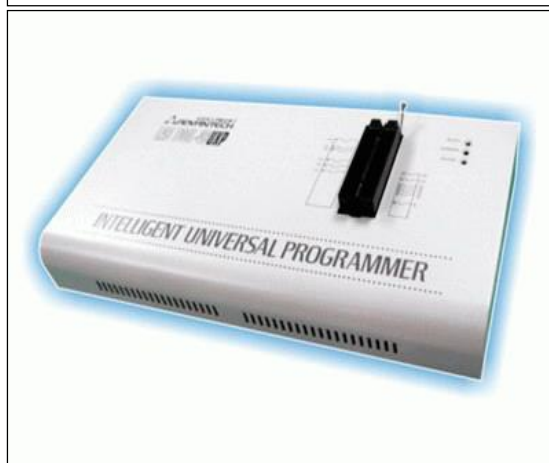
Fig 3: Pin diagram of PIC16F628A microcontroller Fig 4: Intelligent Universal Programmer
